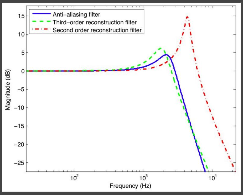
Typical magnitude responses of anti-aliasing filter and reconstruction filters
