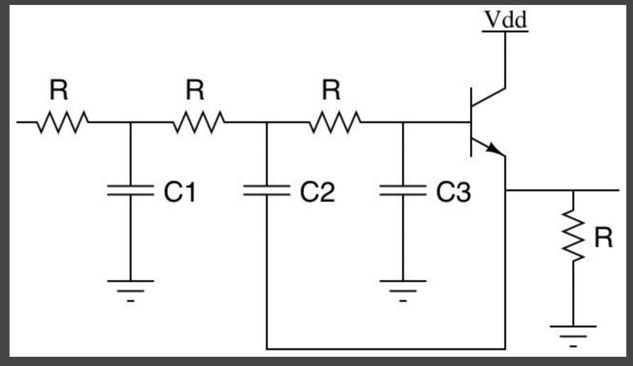
Third-order, transistor-based Sallen-Key low-pass filter
