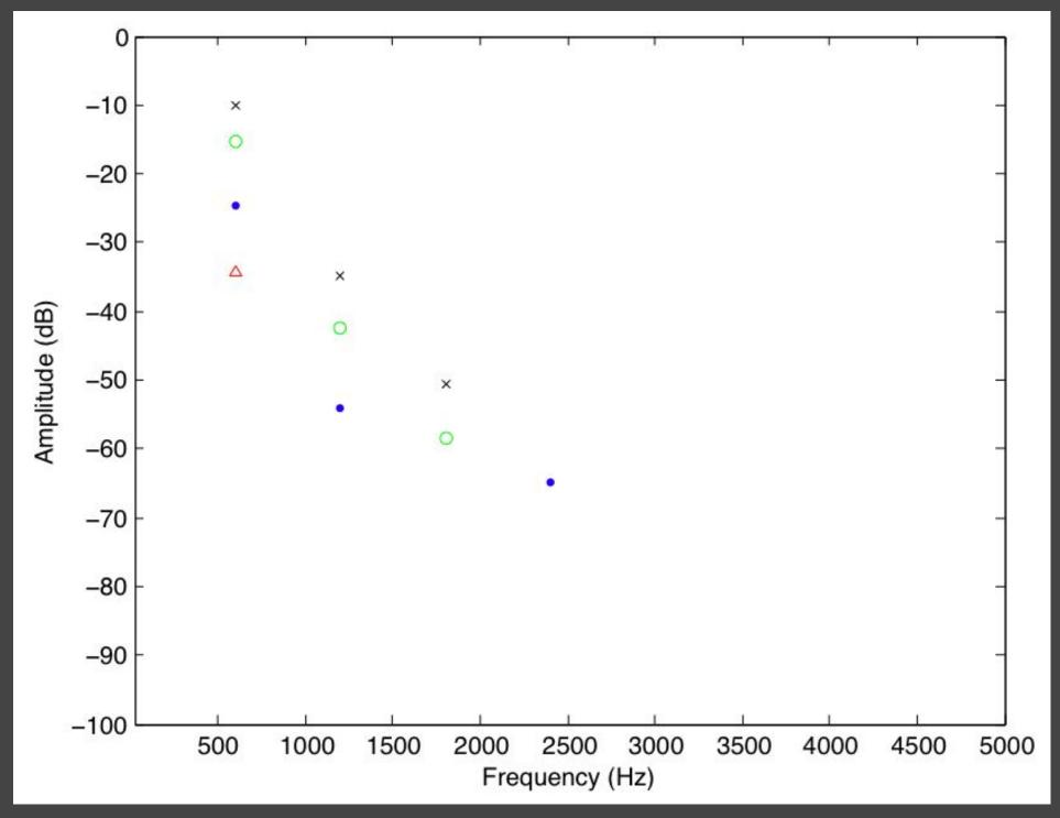
Peaks in magnitude spectrum for pure sine wave inputs at various levels
